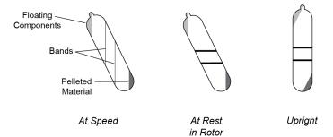
In this example, particles will band about 62 and 64 mm from the axis of rotation, about 2 mm of centerband-to-centerband separation at the rotor's 24-degree tube angle. When the tube is removed from the rotor and held upright (vertical and stationary), there will be about 2.19 mm of centerband-to-centerband separations. This interband distance,  $d_{\rm up}$ , can be calculated from the formula:
