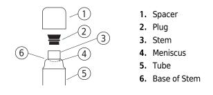
Place the tubes in the rack and fill each tube to the base of the stem, leaving no fluid in the stem.
