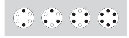
**NOTE** Two, three, four, or six tubes can be centrifuged per run if they are arranged in the rotor as shown. All buckets must be attached to the rotor, whether loaded or empty.
