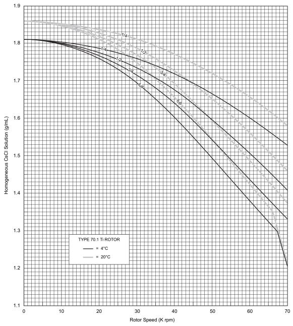
**Figure 2** Precipitation Curves for the Type 70.1 Ti Rotor. Using combinations of rotor speeds and homogeneous CsCl solution densities that intersect on or below these curves ensures that CsCl will not precipitate during centrifugation.
