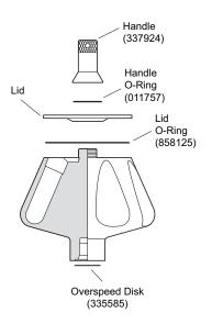
The Type 70.1 Ti, rated for 70 000 rpm, is a fixed angle rotor designed to centrifuge up to twelve tubes at a 24-degree angle to the axis of rotation. Used in Beckman Coulter class H, R, and S preparative ultracentrifuges, the rotor develops centrifugal forces sufficient for applications including pelleting of small particles, and purification of viruses and subcellular organelles using sucrose gradients. Up to 162 mL of sample and gradient can be centrifuged per run.
