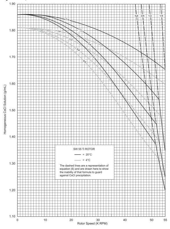
Figure 2 Precipitation Curves for the SW 55 Ti Rotor\*
