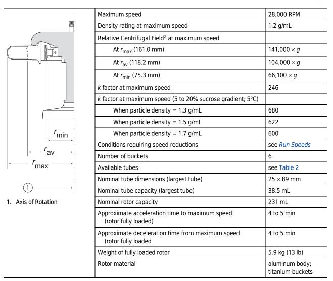
a. Relative Centrifugal Field (RCF) is the ratio of the centrifugal acceleration at a specified radius and speed ( $r\omega^2$ ) to the standard acceleration of gravity (g) according to the following formula: RCF =  $r\omega^2/g$  — where r is the radius in millimeters,  $\omega$  is the angular velocity in radians per second (2  $\pi$  RPM /60), and g is the standard acceleration of gravity (9807 mm/s<sup>2</sup>). After substitution: RCF = 1.12r (RPM/1000)<sup>2</sup>
