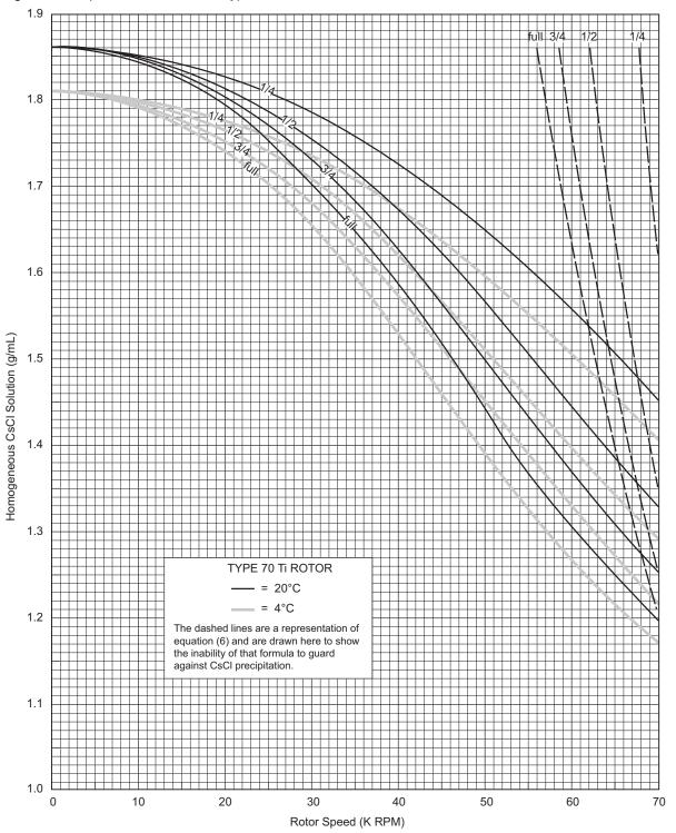
Figure 6 Precipitation Curves for the Type 70 Ti Rotor\*
