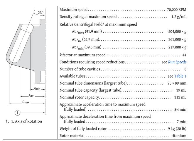
a. Relative Centrifugal Field (RCF) is the ratio of the centrifugal acceleration at a specified radius and speed ( $r\omega^2$ ) to the standard acceleration of gravity (g) according to the following formula: RCF =  $r\omega^2/g$  — where r is the radius in millimeters,  $\omega$  is the angular velocity in radians per second (2  $\pi$  RPM /60), and g is the standard acceleration of gravity (9807 mm/s<sup>2</sup>). After substitution: RCF = 1.12r (RPM/1000)<sup>2</sup>
