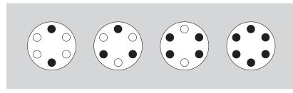
**NOTE** Two, three, four, or six tubes can be centrifuged per run if they are arranged in the rotor as shown. All buckets must be attached to the rotor, whether loaded or empty.
