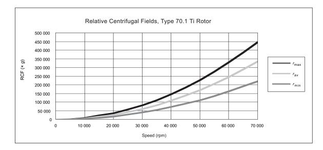
**2.** *Further speed limits must be imposed* when CsCl or other self-forming-gradient salts are centrifuged, as EQ 6 does not predict concentration limits/speeds that are required to avoid precipitation of salt crystals. Solid CsCl has a density of 4 g/mL, and if precipitated during centrifugation may cause catastrophic rotor failure and instrument damage. Figure 2 and Figure 3, together with the description and examples below, show how to reduce run speeds when using CsCl gradients.
