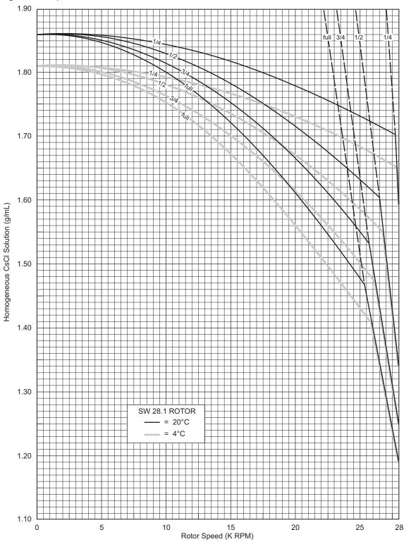
Figure 4 Precipitation Curves for the SW 28.1 Rotor\*
