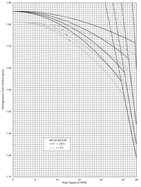
Figure 2 Precipitation Curves for the SW 28 Rotor\*
